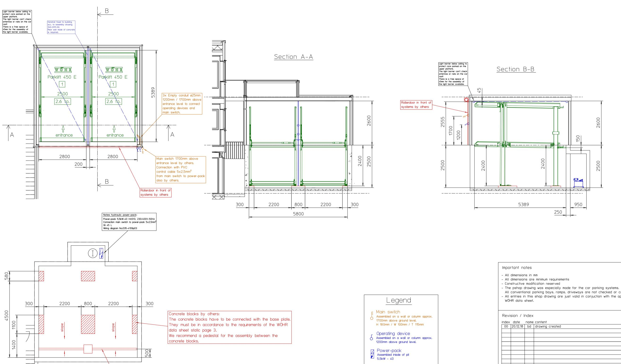
Pump-sump, slope and drainage
